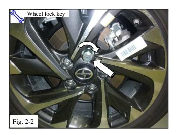
(b) Take the key supplied in the wheel lock set and place it on top of the wheel lock. Turn the key until the patterns engage (Fig. 2-2).
